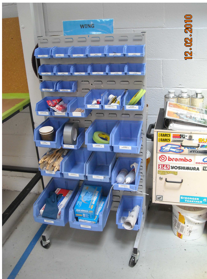
Mobile parts 'supermarket' right next to workstation replacing old stores setup that people spent hours each day going to and from.
